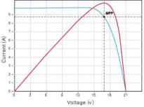
The MPPT point under changing light intensity and temperature of environment. The MPPT controller could adjust the MPP timely according to different conditions.
